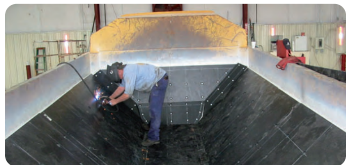
Strongly anchored: Installation or Matrox sheets in a funnel-shaped dump truck using the stud-welding process
